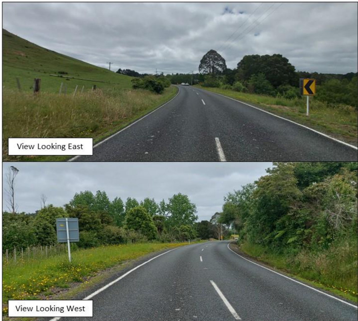
Figure 5: Ararimu Road Indicative Sight Distance toward Vehicle Crossing
